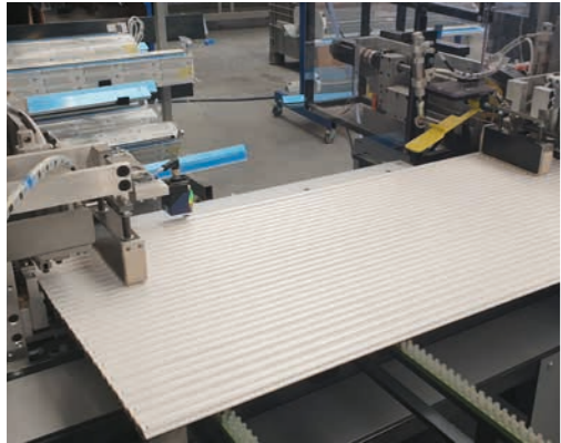
Machine for cutting and assembling aluminium roller shutter apron
