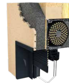
FoKus 235 box Timber frame assembly ALU bioclimatic slat anthracite grey 7016
